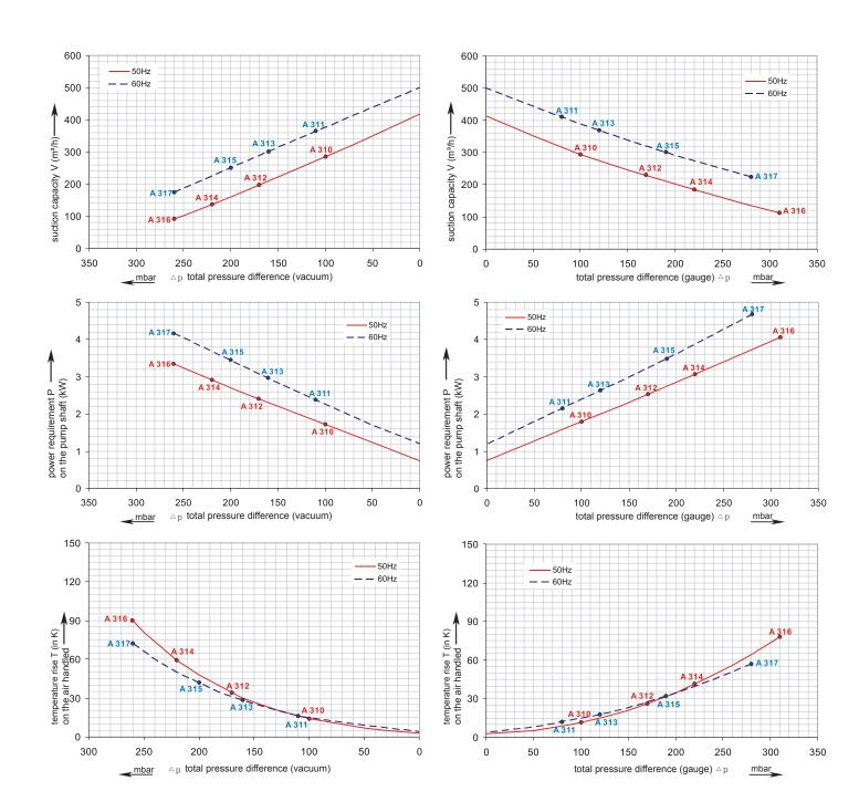
The performance curves are based on air at a temperature of 15  $^{\circ}C$  and an atmospheric pressure of 1013 mbar with a tolerance of +/- 10 %. The total pressure differences are valid for suction and ambient temperatures up to 25  $^{\circ}C$ .
