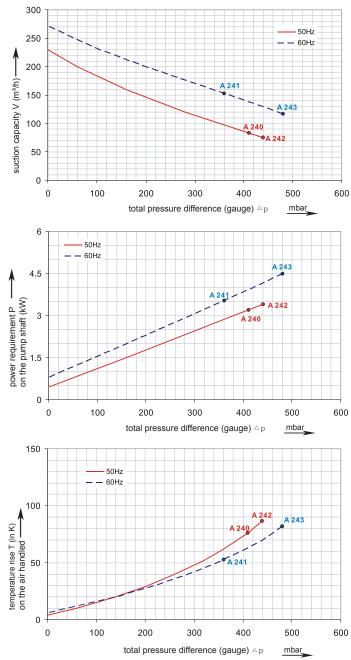
The performance curves are based on air at a temperature of 15 °C and an atmospheric pressure of 1013 mbar with a tolerance of +/- 10 %. The total pressure differences are valid for suction and ambient temperatures
