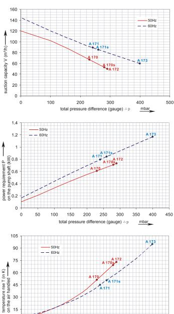
The performance curves are based on air at a temperature of 15 °C and an atmospheric pressure of 1013 mbar with a tolerance of +/- 10 %. The total pressure differences are valid for suction and ambient temperatures up to 25 °C.
