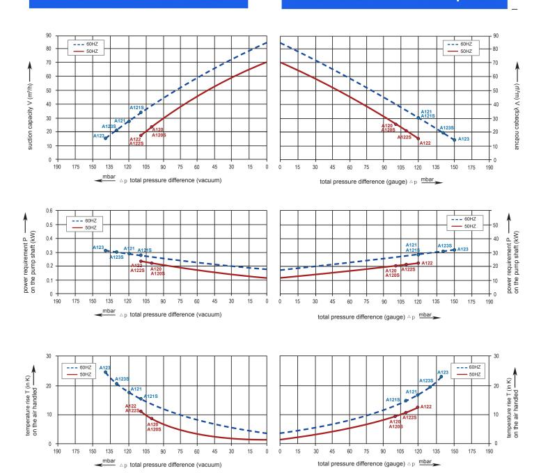
The performance curves are based on air at a temperature of 15 °C and an atmospheric pressure of 1013 mbar with a tolerance of +/- 10 %.
